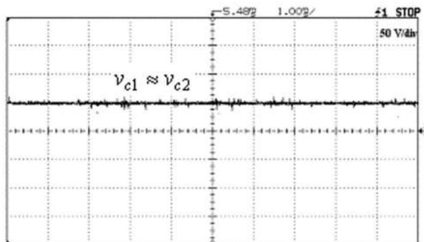
Fig. 13. Equalized voltage due to chopper action.
