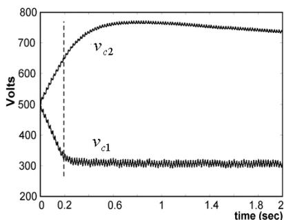
Fig. 5. Voltage imbalance in capacitors.
