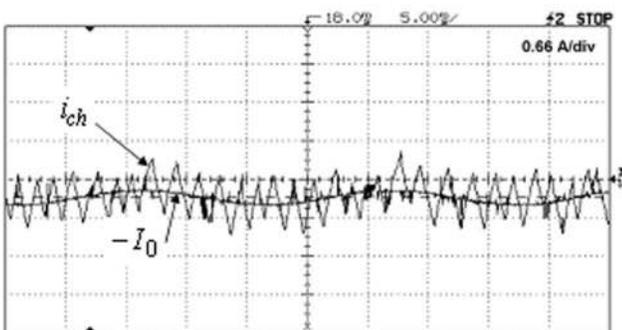
Fig. 12. Chopper current using hysteresis control: Experimental.
