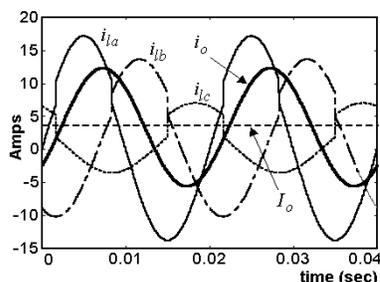
Fig. 4. Load currents with dc component.
