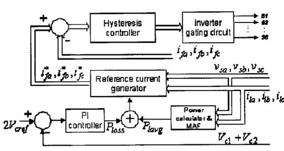
Fig. 2. Control scheme for VSI operating as current source.
