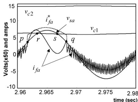
Fig. 6. Effect of dc component of load on tracking performance.
