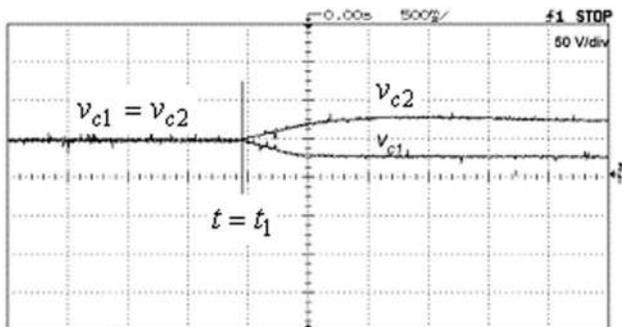
Fig. 10. Voltage imbalance in capacitors: experimental.
