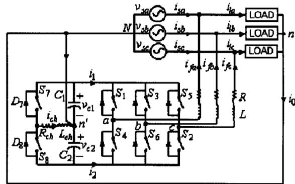
Fig. 1. Compensator for star-connected three-phase, four-wire distribution system.
