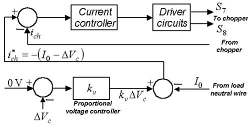
Fig. 3. Schematic of chopper control.
