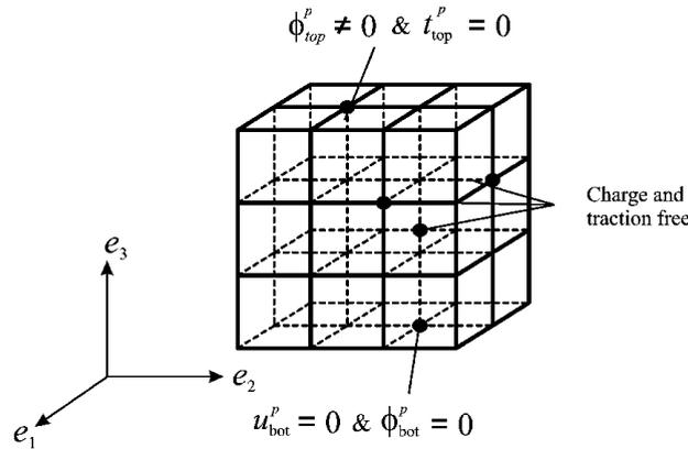
Fig. 5. Boundary conditions applied to the finite element discretization of the block-like specimen.
