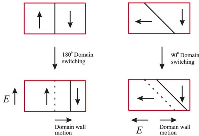
Fig. 3. Two-dimensional graphical illustration of domain wall motion.
