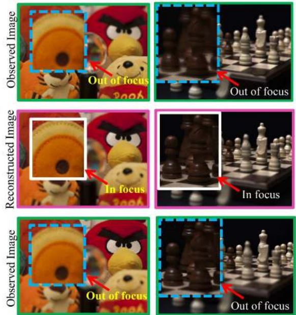
Figure 12: Focal Aperture Stack Reconstruction of an unobserved focal-aperture setting. 16 images with varying focus and aperture settings given by our optimal sampling scheme are captured and the entire epsilon photography stack is reconstructed. (middle row) An example of a reconstructed image with zoomed in insets for two datasets. (top, bottom) Two observed images that are closest in focus and aperture settings to the one in the middle row. The reconstruction shows ability to transfer textural detail and sharpness to unobserved focal-aperture settings.
