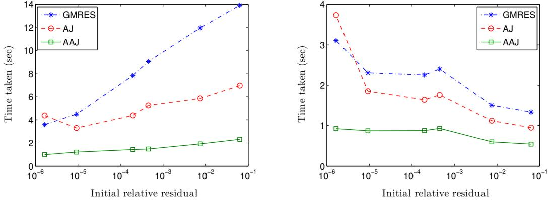
(a) Convergence to a tolerance of  $\epsilon = 1 \times 10^{-8}$ . (b) Initial relative residual reduction by a factor of 0.01.
