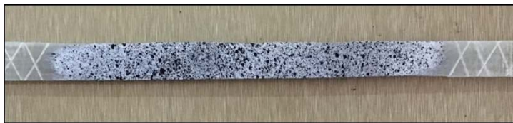
Figure 2. Tensile Test specimen — 0^\circ fibre orientation
