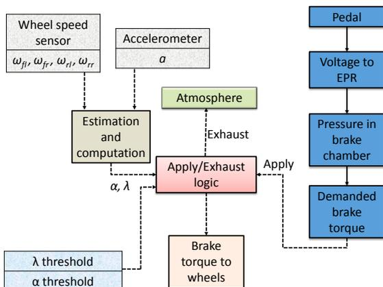
Fig. 4. Block diagram of Apply-Exhaust Logic
