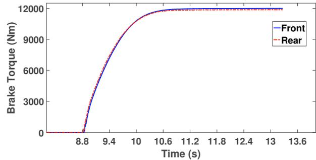
Fig. 5. Open loop panic brake torque applied
