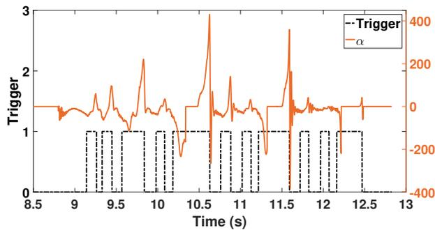
Fig. 15. Wheel acceleration response for front wheels where  $\lambda_{th} = 12\%$
