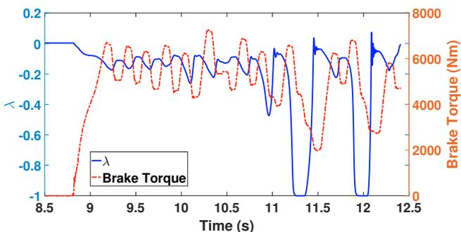
Fig. 16. Slip regulation for front wheels where  $\lambda_{th}=12\%$ ,  $\alpha_l=-40$  rad/s<sup>2</sup> and  $\alpha_h=+40$  rad/s<sup>2</sup>
