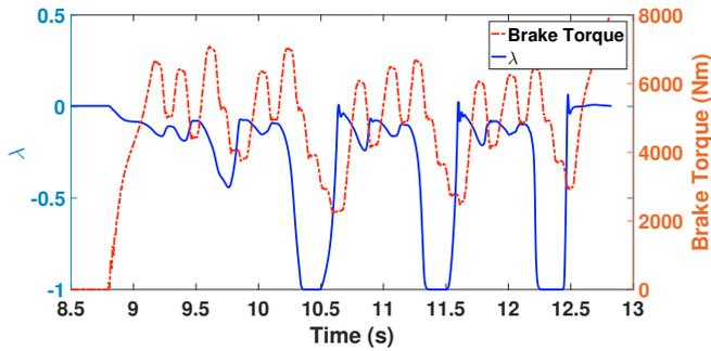
Fig. 14. Slip regulation for front wheels where  $\lambda_{th} = 12\%$
