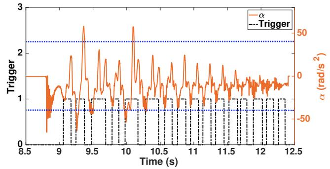
Fig. 11. Wheel acceleration response for front wheels where  $\lambda_{th} = 9 \%$
