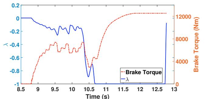
Fig. 9. Slip regulation for front wheels where  $\alpha_l = -20 rad/s^2$
