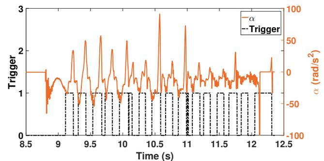
Fig. 13. Wheel acceleration response for front wheels where  $\lambda_{th} = 10 \%$
