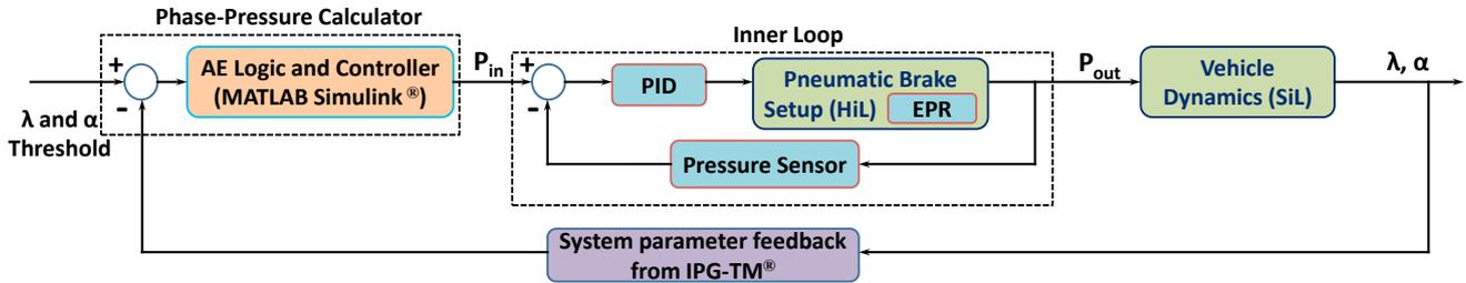
Fig. 2. Block level diagram of the control loops involved in threshold analysis
