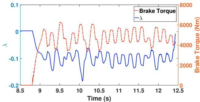
Fig. 10. Slip regulation for front wheels where  $\lambda_{th} = 9 \%$
