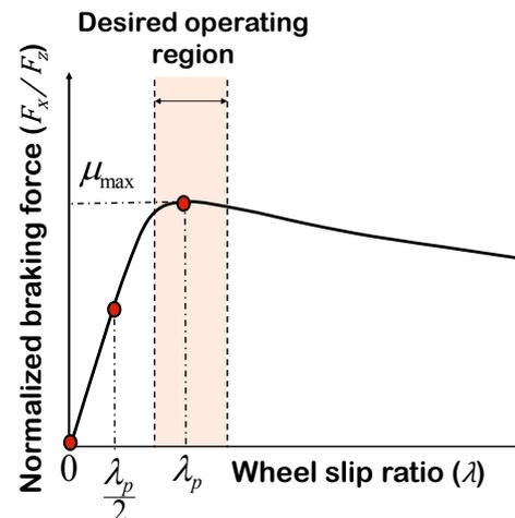
Fig. 1. Normalized braking force - wheel slip curve
