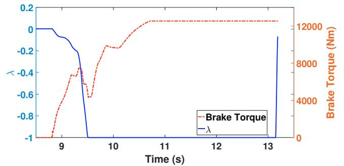
Fig. 7. Slip regulation for front wheels where  $\alpha_l = -40 rad/s^2$
