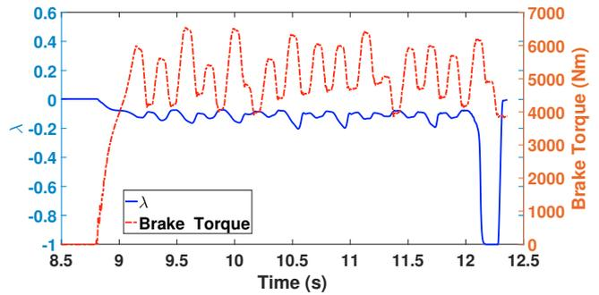
Fig. 12. Slip regulation for front wheels where  $\lambda_{th} = 10 \%$
