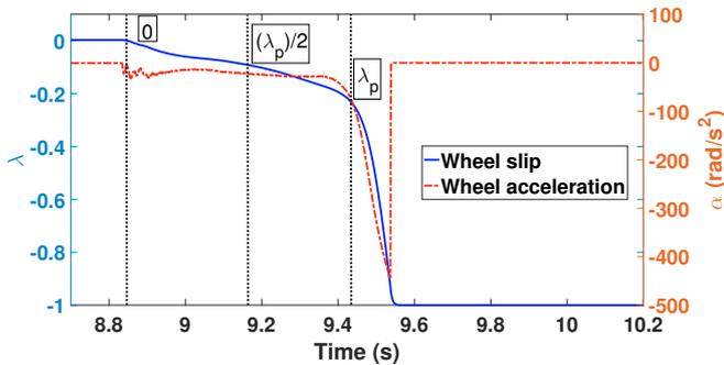
Fig. 6. Open loop response for front wheel
