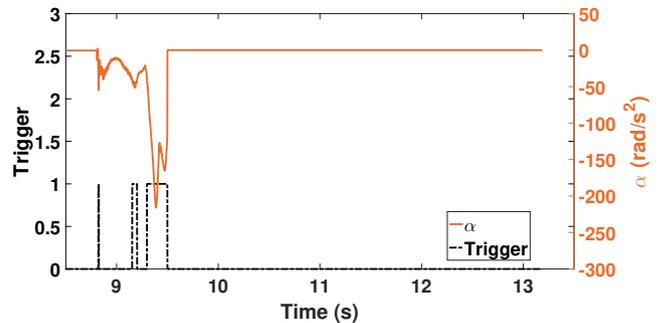
Fig. 8. Wheel acceleration response for front wheels where  $\alpha_l = -40 rad/s^2$
