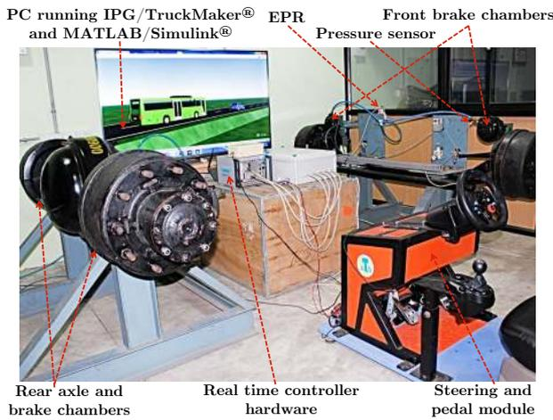
Fig. 3. HiL setup used for experimentation
