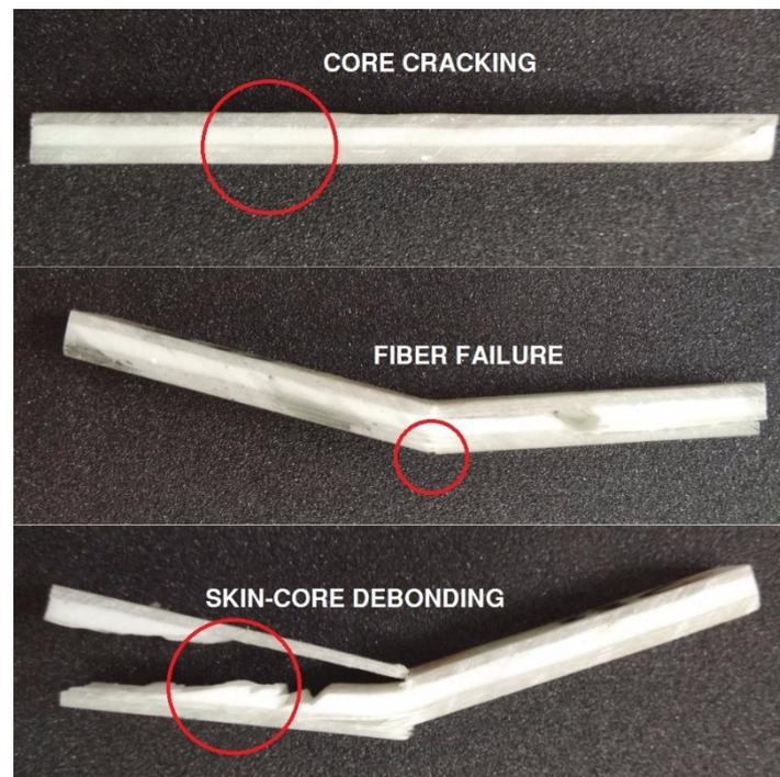
**Figure 3.** The stages involved in flexural failure of syntactic foam - GFRP sandwich composites.
