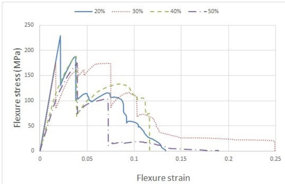
**Figure 4.** The flexural stress-strain curves of sandwich composites with varying foam volume fraction (core thickness equal 3 mm).
