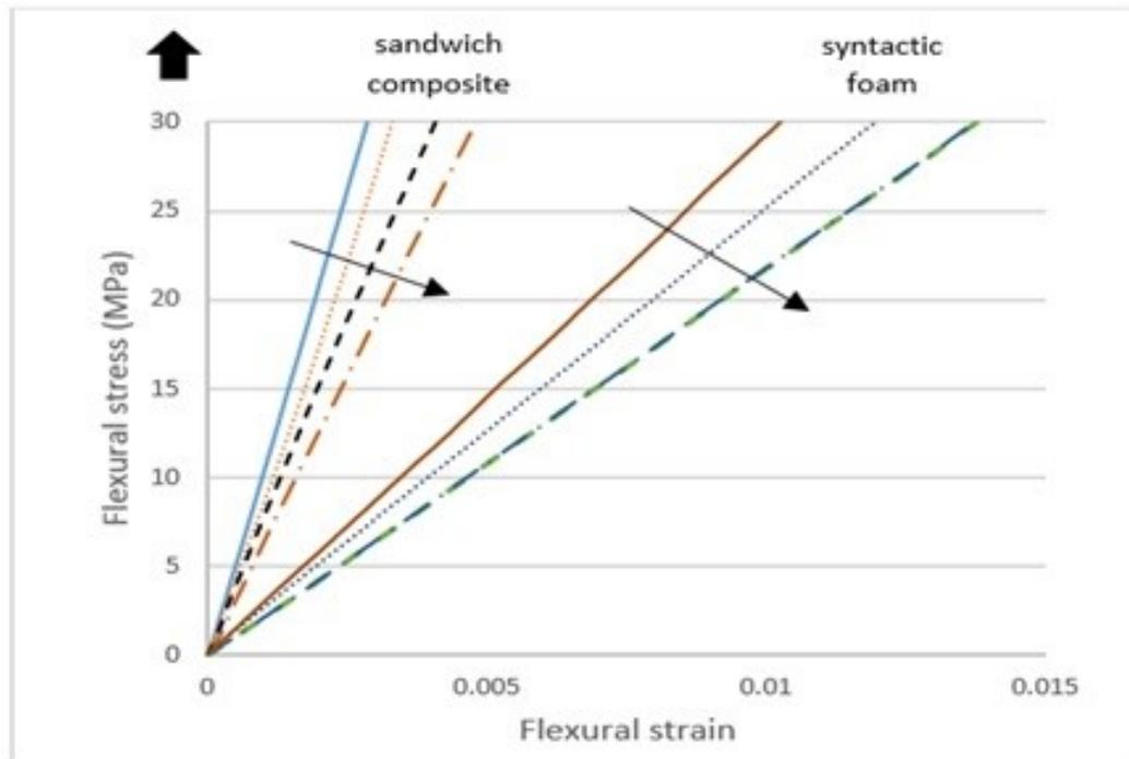
**Figure 5.** The initial portion of the flexural stress-strain curve compared with pure syntactic foam curves. The arrows depict increasing core volume fraction.
