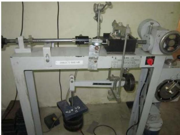
**Fig. 4** The direct shear pull out test setup
