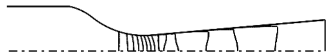
Figure 14 Contours of |1 - Z| in the primary nozzle corresponding to a generator temperature of 103°C
